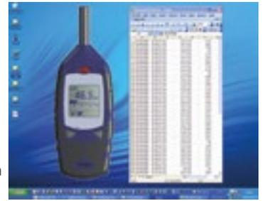
spreadsheet applications. Data stored within the 24x series can also be accessed since these meters act like a memory stick, allowing transfer of data to spreadsheet applications.
