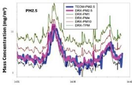
Comparison of Arizona Road Dustriess concentration measured by the DustTrak DRX and the TEOM with a PM2.5 impactor.
